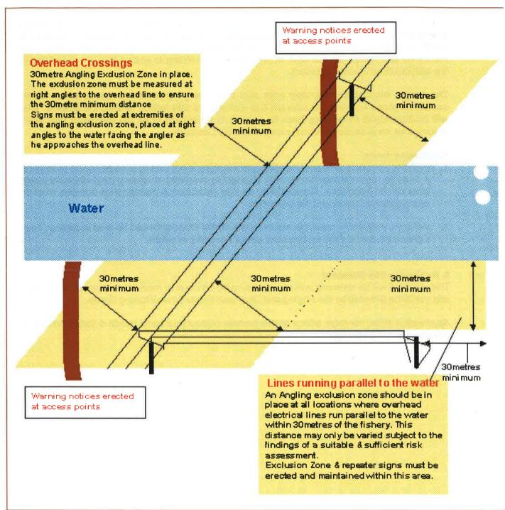
**Application Note:** The measurements must be taken along the ground at right angles to the outer conductor of the overhead power line.
